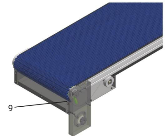
9 CONVEYOR MAINTENANCE - TENSIONING & GREASING OF DRIVE CHAIN
