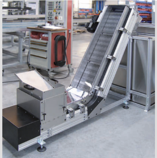
KFS-P 2040.86 for hot product with resizeable supply reservoir
