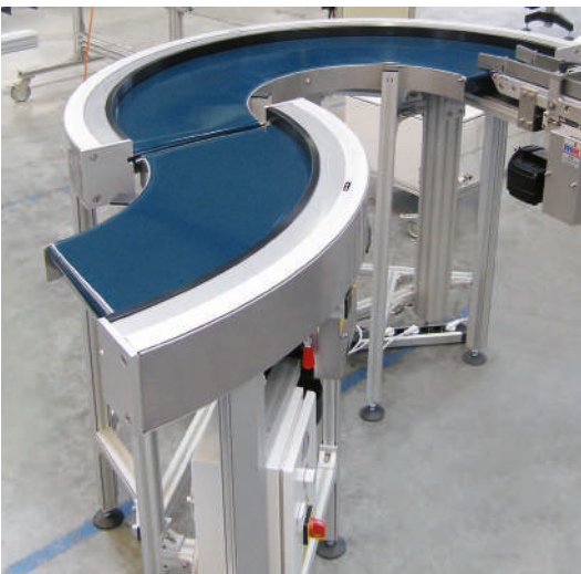
Combination of 90° and 180° KGF-P 2040 curved belt conveyors with lower belt drive BI, reversible
