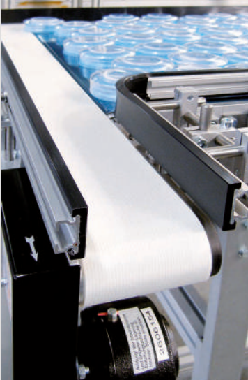
GUF-P 2000 as cross conveyor and separator
