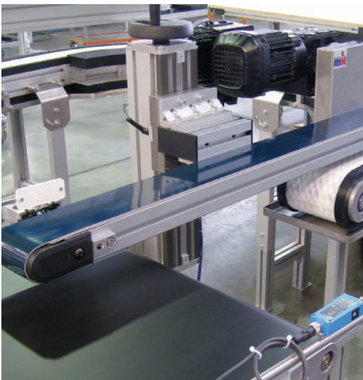
VST 2011-H with handwheel as add-on kit for the belt conveyor with incline adjustment
