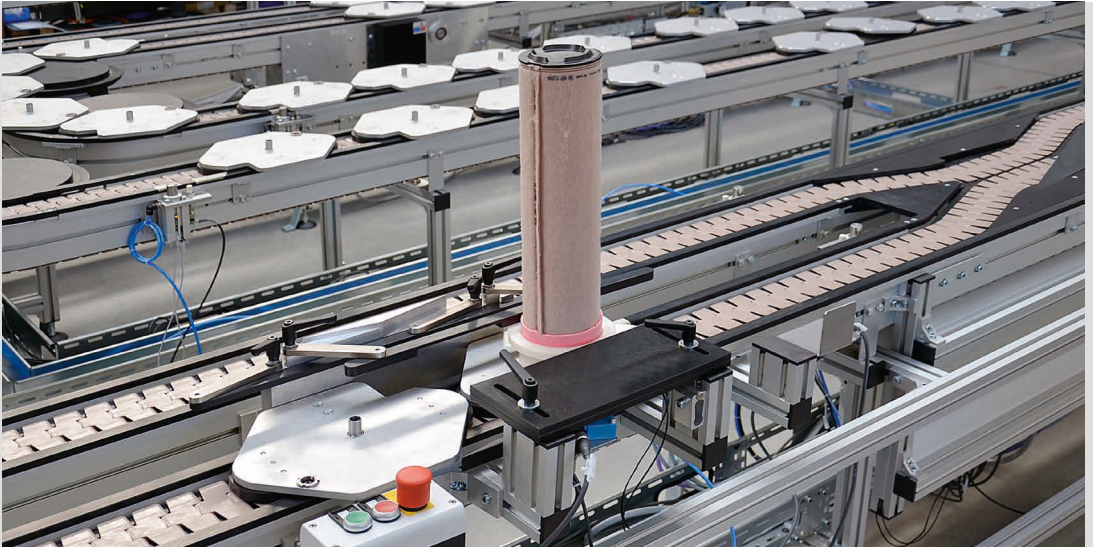
SBF-P 2254 as an interlink with a removal and loading station for pallet holders
