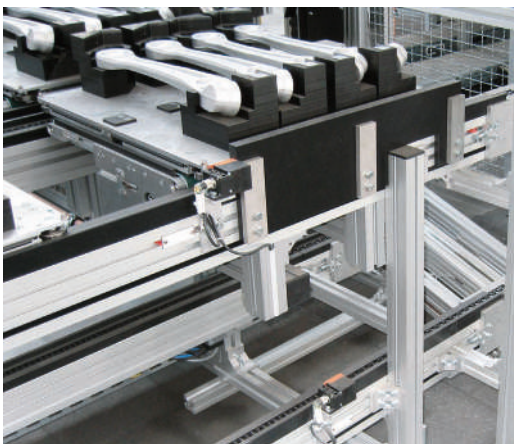
Foolproof part pickup for left-sided and right-sided products
