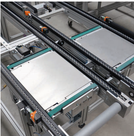
Lift-and-transfer conveyor in parallel arrangement with support roller for bridging small gaps
