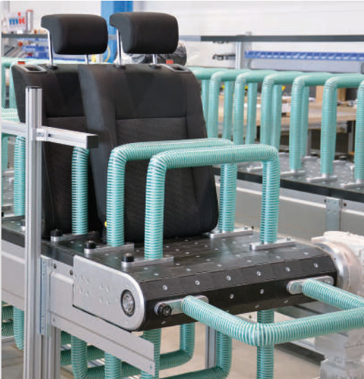
Cycled modular belt conveyor with bolted-on tubular brackets in a special design
