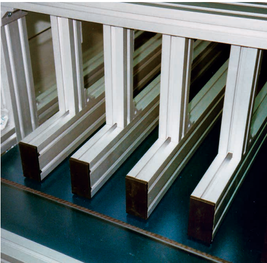
Multi-line, adjustable side rail in gantry arrangement
