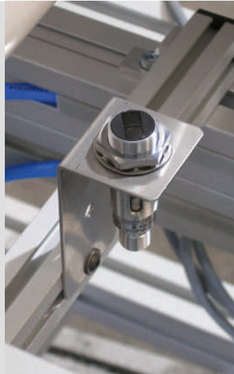
Initiator holder made from VA steel sheet
