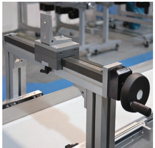
Manual two-axis adjustment system for holding a marking device with VST 2015
