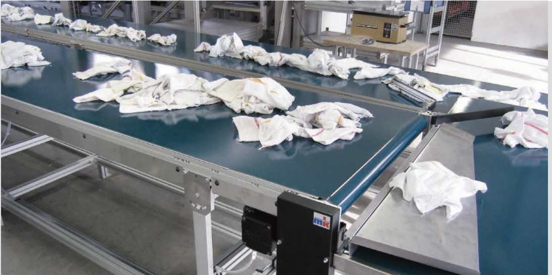
Circulation system for manually sorting laundry based on GUF-P 2041 and GUF-P 2000 conveyors with AC head drive
