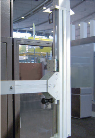
Electromotive VST 2015 with recirculating ball bearing guide
