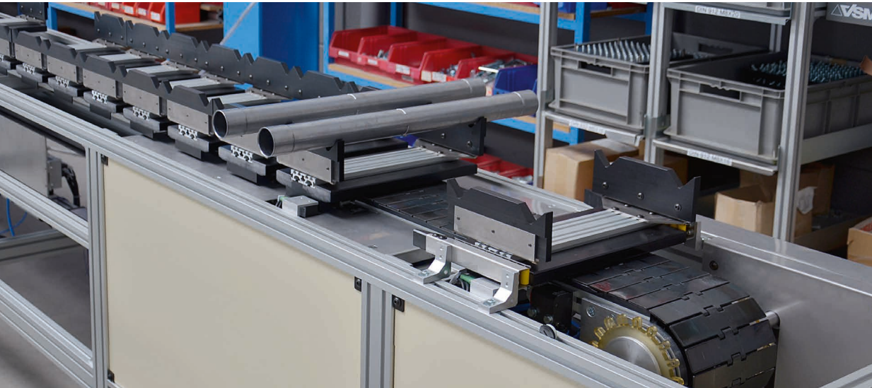
SPU accumulating pallet circulation system with pallet separation function as a feed for parts for a production system
