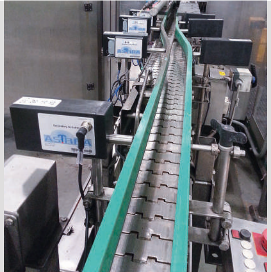
SBF EMMA stainless steel conveyor with automatically adjustable side rail ASTRA
