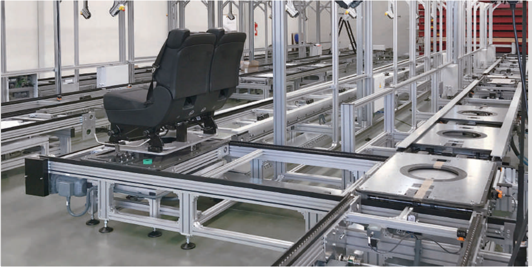
Versamove plus with large custom pallets
