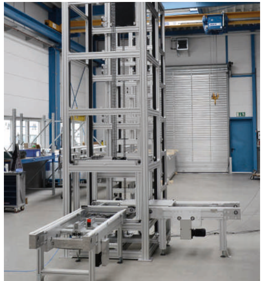
Lift that is accessible from three sides, with rotating assembly in the lift carriage and feed via a Versamove ultra
