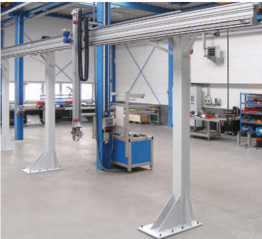
X-Z gantry with gripper for transferring crankshafts. X axis as LZR with support roller and timing belts, Z axis with timing belt Omega drive and fall arrest
