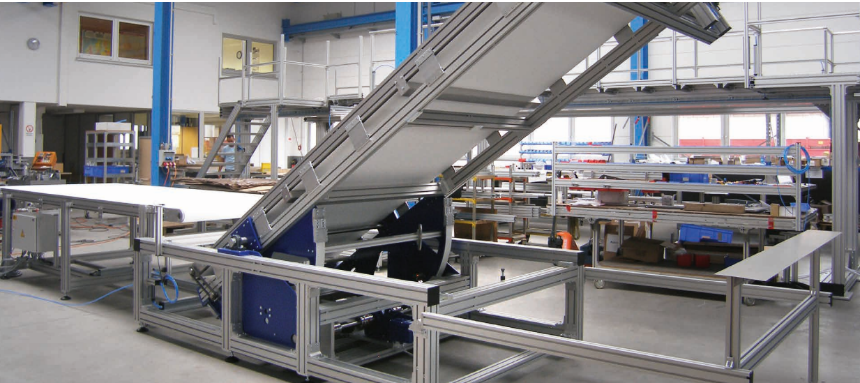
Pivoting conveyor system with integrated slug clamping, that picks off and clamps blow moulded parts on the machine and transports them away.
