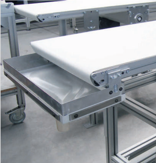
Belt conveyor with dust bag
