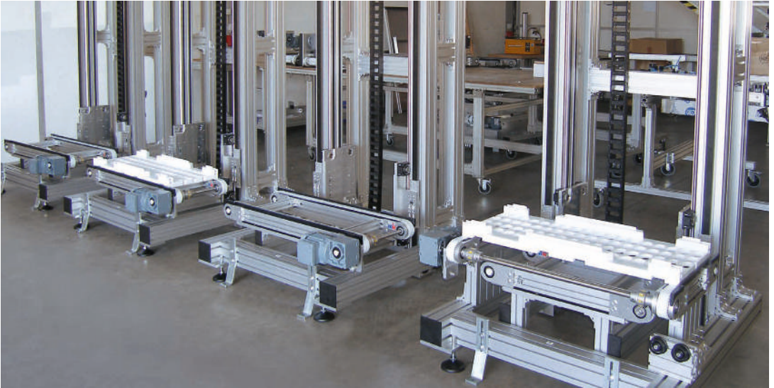
Dual LZR 2005-38.44 with cantilever for dual ZRF-P 2010 for lift and transfer from a dual ZRF-P as a lift-and-transfer module
