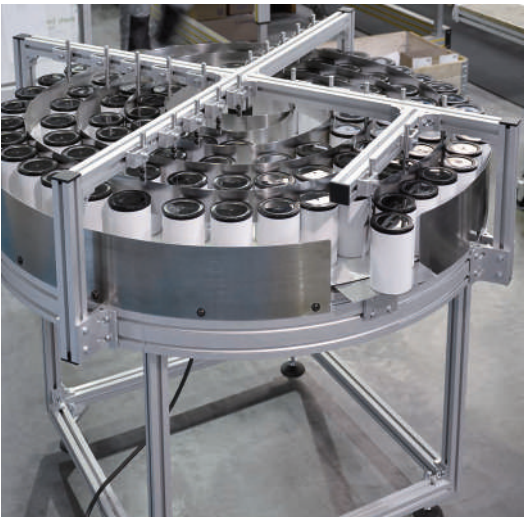
Rotary table with additional custom add-on
