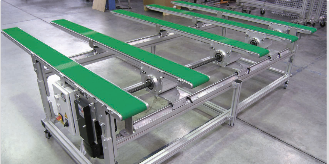
GUF-P MINI with lower belt drive BC as special configuration with 5 conveying lines. The inner conveying lines can be moved manually and are guided by guide rods
