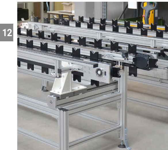
TKU 2040 with special adjusting unit for adjusting the distance between the conveyor chains
