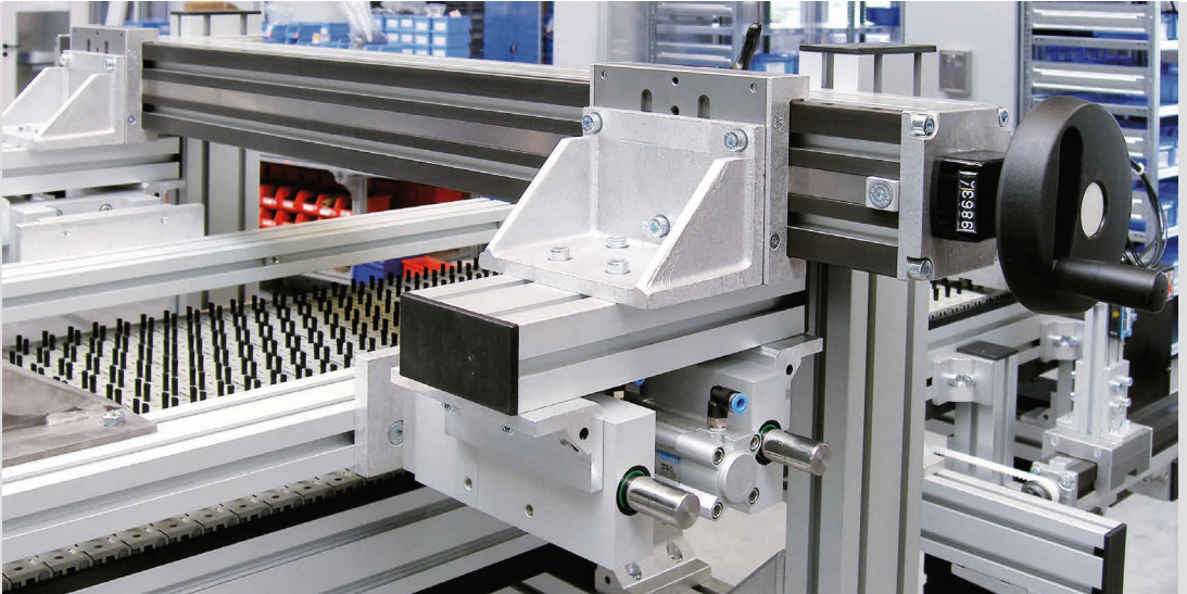
VST 2011 with two counter-rotating slide carriages and digital display for adjusting the width of the pneumatic centring unit on the modular belt conveyor
