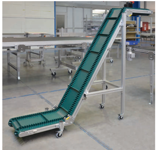
KFG-P 2000 ECO with head drive AF and 60° incline variant B3 (B20.00.015-B3)
