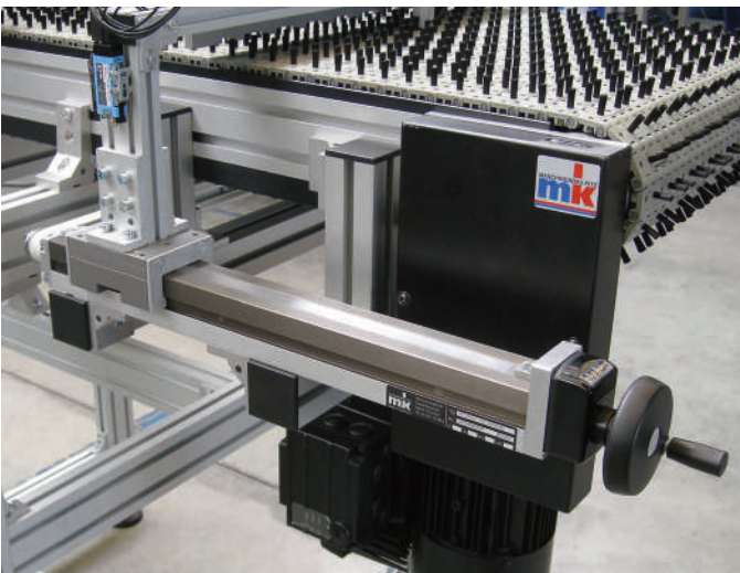
Dual VST 2015 with manual digital display for adjusting the stop bar
