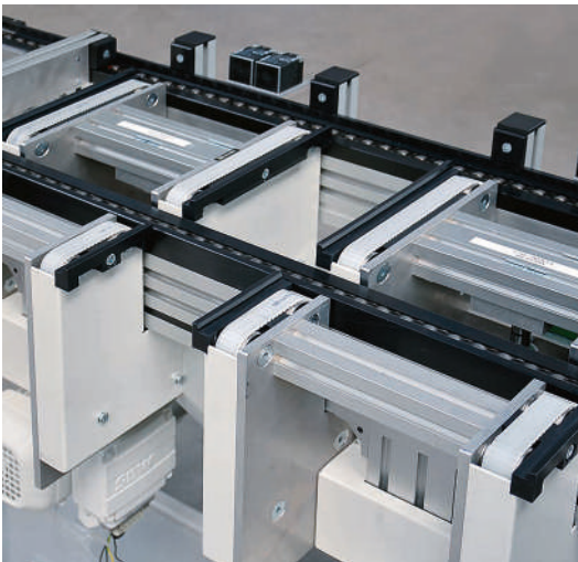
Lift-and-transfer conveyor with coupled drive and central stroke unit for bridging very short transverse sections
