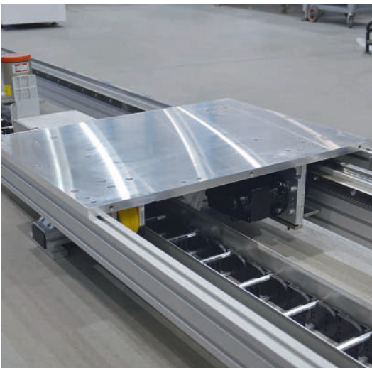
Transfer shuttle with pallet carriers, carriage with recirculating ball bearing guide
