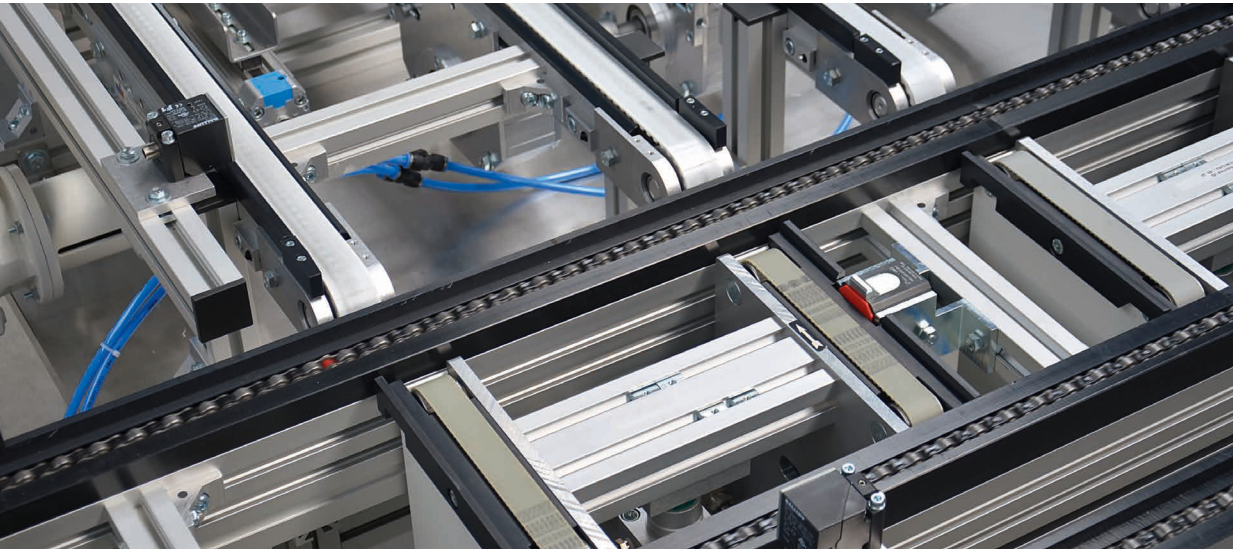
Separation of pallets from the main line in two parallel cross conveyor tracks
