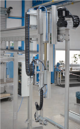
Gantry stand with telescopic gripper unit
