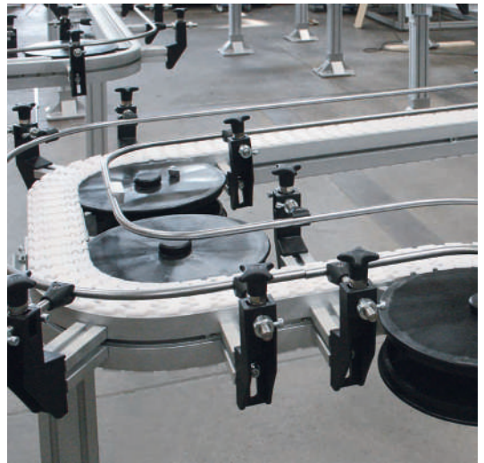
SBF EMMA with rolling curves and side rails
