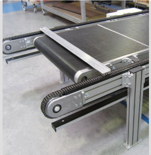
Combination of belt conveyor and chain conveyor with transverse rail for simulating a floor obstacle
