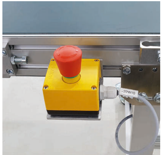
Emergency stop button
