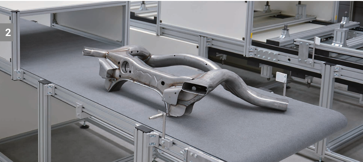
GUF-P 2041 with protective tunnel as discharge belt for rear axle parts
