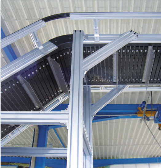
Solid support of the KFS-P 2040.86 for conveying heavy loads
