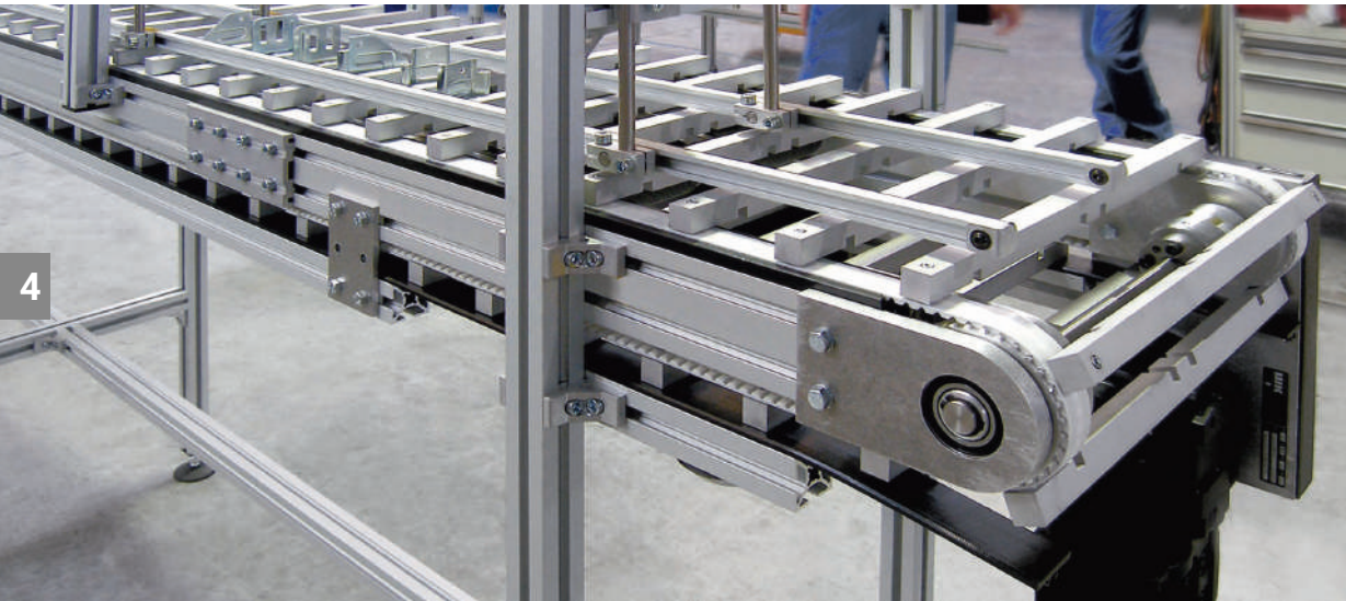
ZRF-P 2040, threaded sleeves integrated into the timing belt enable customer-specific cams to be bolted on
