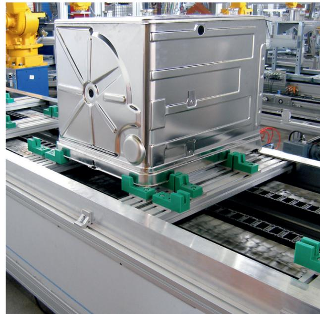
A SPU 2040 wide unit is used as an infeed conveyor for dishwasher units.
