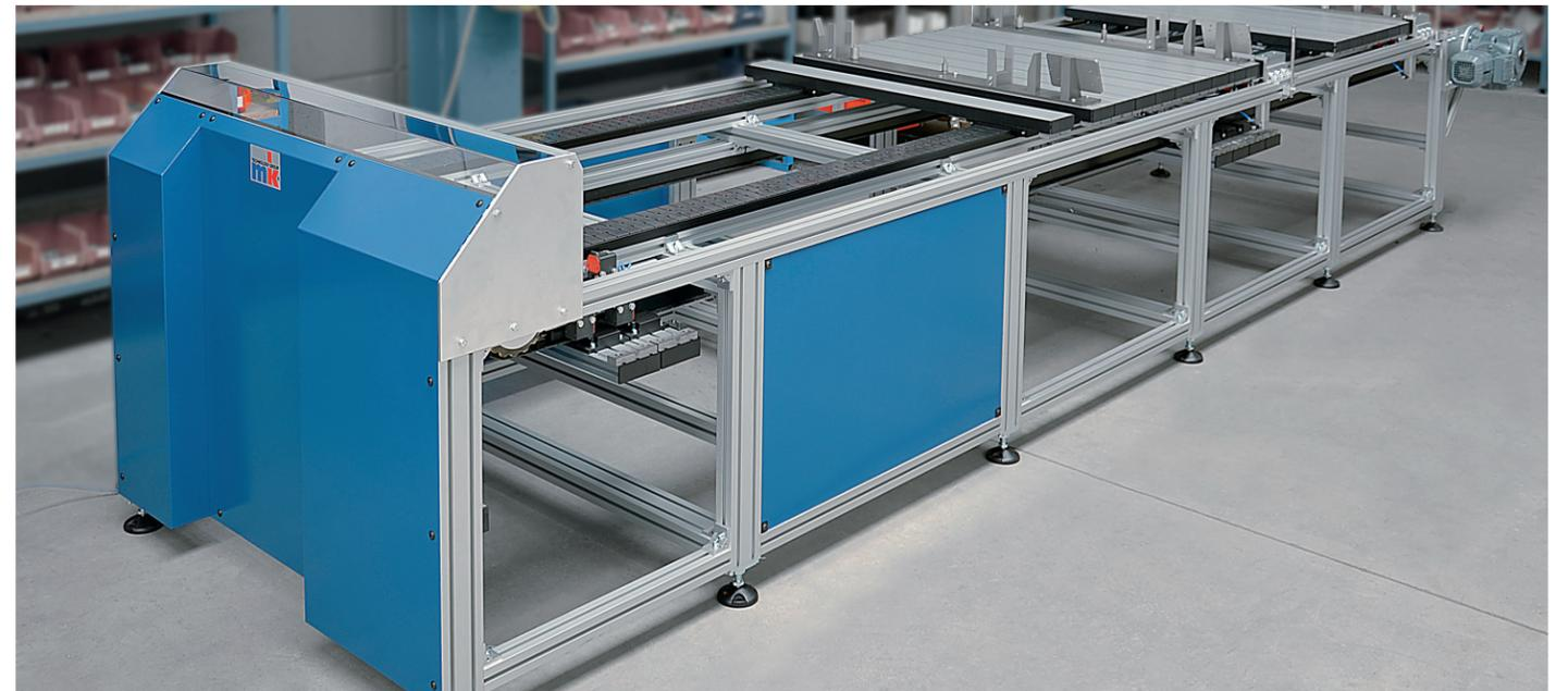
A wide SPU 2040 for supplying parts in an assembly and welding facility
