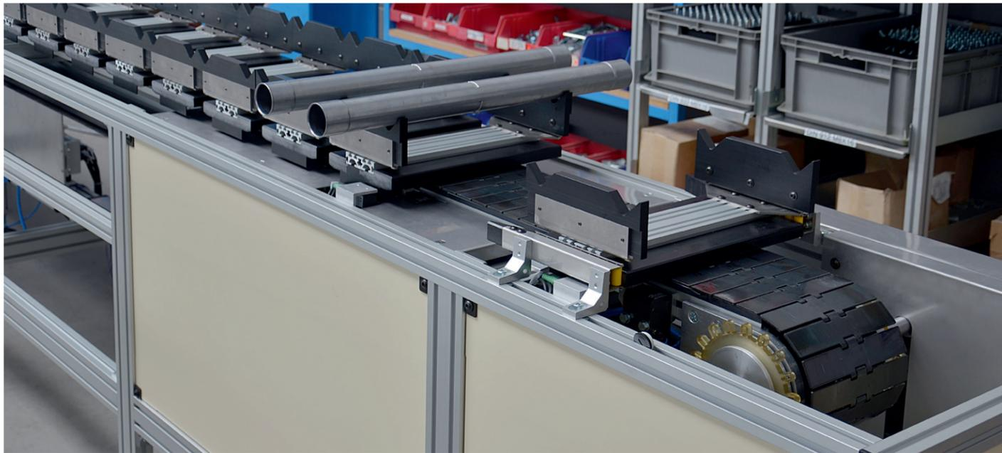
A SPU 2040, with pallet separating function (pallet singulator) for supplying parts in a production facility.
