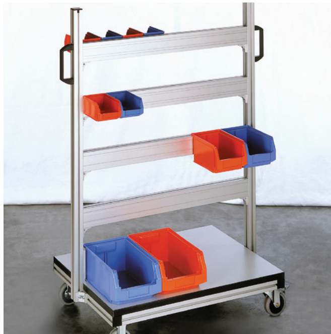
Carts can be designed to be accessible from two or more sides, and are excellent for holding work-in-progress materials.
