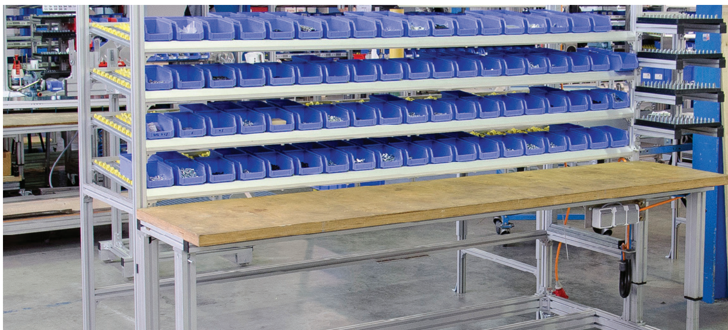
Plastic bins can neatly and effortlessly be stored on a workbench, and fed to the work space via roller racks.
