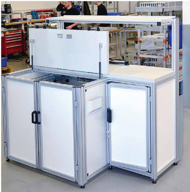
Storage containers can be made as simple or as complex as the need requires. Swinging doors, as well as lift-top access, are all feasible.
