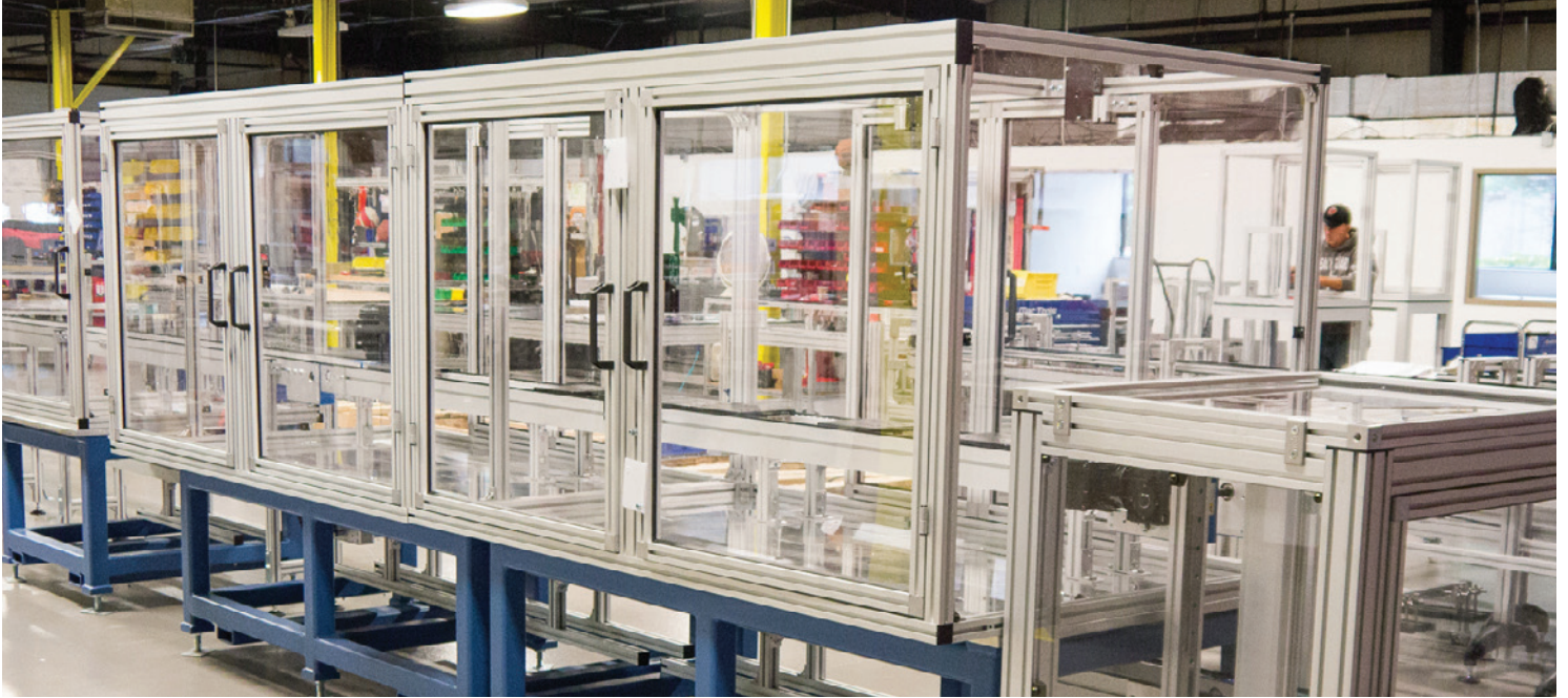
Polycarbonate paneling makes it easy to see what is happening within a work cell, and swinging doors makes it easy to access the inside of the cell.
