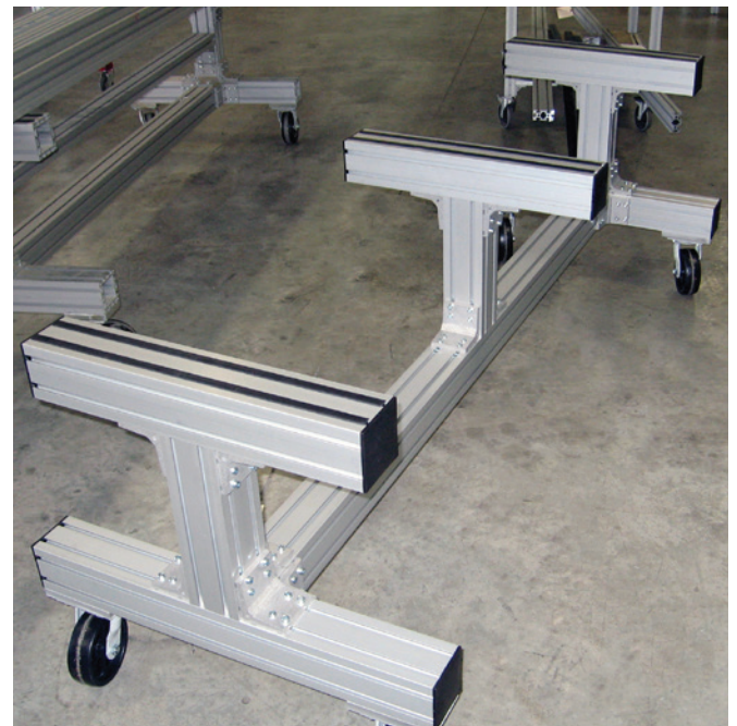
Because mk extrusion comes in a variety of sizes, workhorses can be designed to take as much or as little load as called for,
