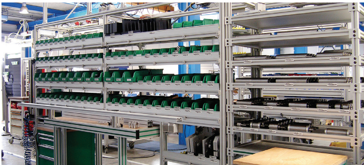
Kanban workstations can be configured to match the process and area they are installed in.
