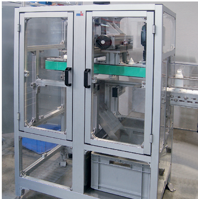
Polycarbonate paneling is an excellent choice when seeing inside a work cell is paramount. Polycarbonate comes both clear and tinted.
