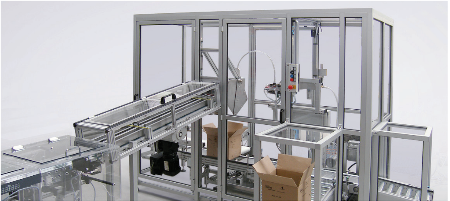
Machine guarding can be used to tie various pieces of equipment and processes together; providing a cohesive and safe design.
