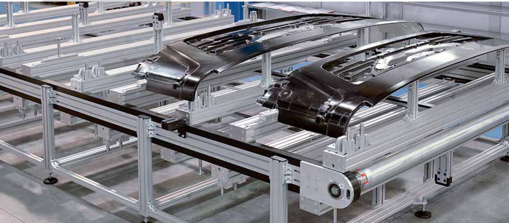
A wide width TKU 2040 with Profile Pallets, complete with locating fixtures for the automotive industry.
