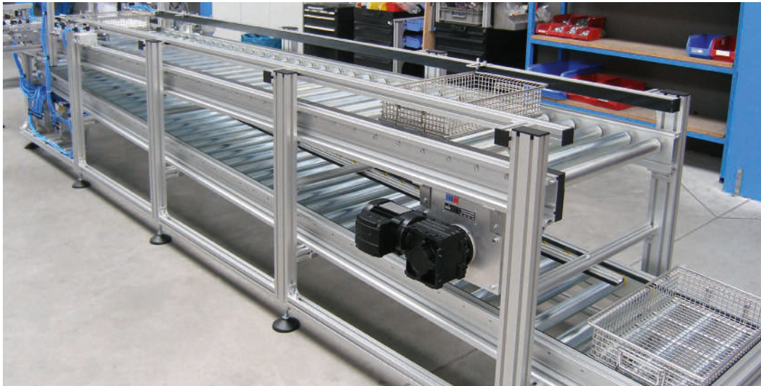
Friction roller conveyor RBT-P 2255 with oscillating conveyor operating as a lift for returning empty baskets
