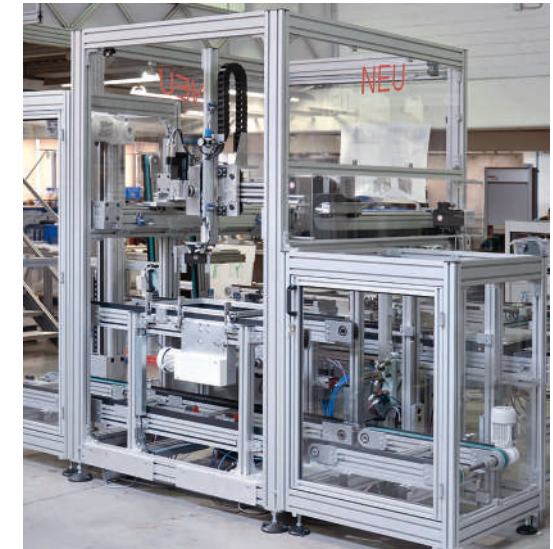
Pallet circulation system for various transport levels with three-axis gantry
