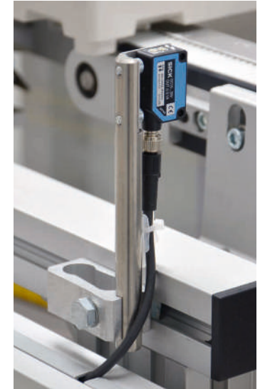
Photoelectric sensor with adjustable holder
