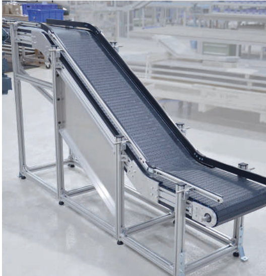
Incline conveyor KFM-P 2040 with side rail, guide rail type 22
