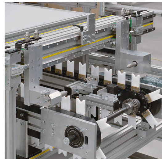
TKU 2040 for transporting camshafts with positioning sensors
