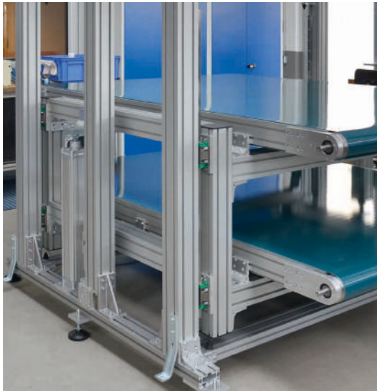
Lift station for lifting and lowering conveyors on two conveyor levels. Cross-conveyor unit with recirculating ball bearing guides positioned horizontally in the frame
