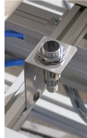
Initiator holder made from VA steel sheet
