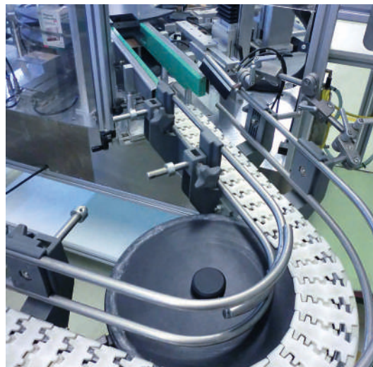
Versaflex flat top chain conveyor with wheel bend and side rail
