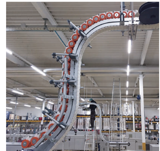
Versaflex SBF with pressure rollers for vertical transport
