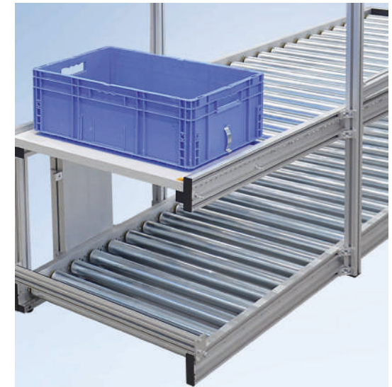
Gravity roller conveyor RBS-P 2066 with ø 50 steel rollers as supply and return line with shelf at the end of the conveyor
