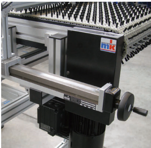
Dual VST 2015 with manual digital display for adjusting the stop bar
