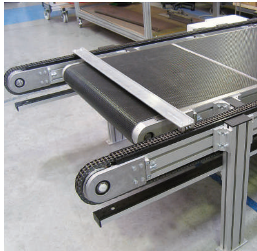
Combination of belt conveyor and chain conveyor with transverse rail for simulating a floor obstacle
