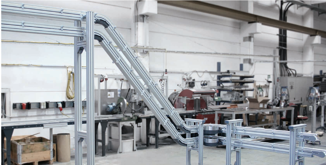
Versaflex SBF A06 with flat top chain with cams for vertical transport
