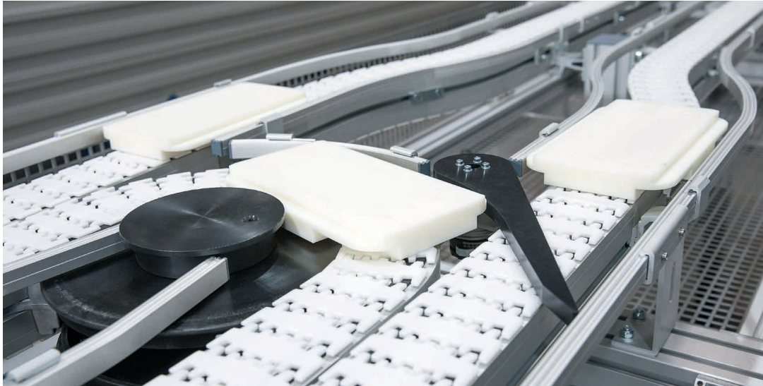
Pallet system based on SBF Versaflex A08 with separator
