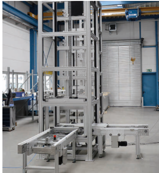
Lift that is accessible from three sides, with rotating assembly in the lift carriage and feed via a Versamove ultra
