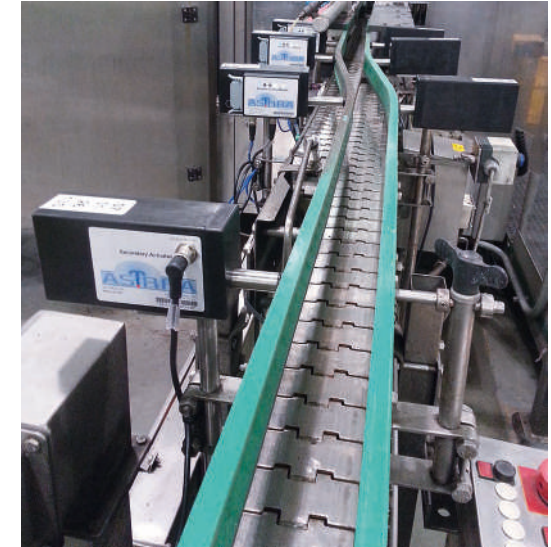
Versaflex SBF stainless steel conveyor with automatically adjustable side rail ASTRA
