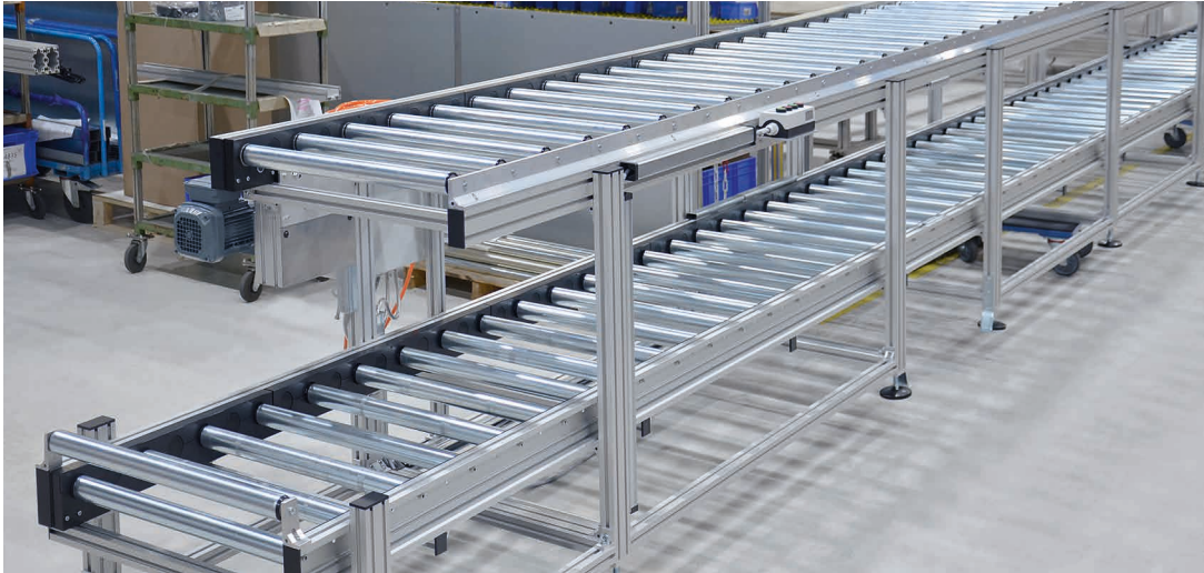
Tangential chain roller conveyor RBT-P 2255 for continuous and accumulated operation with test parts
