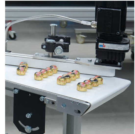
GUF-P 2000 with rolling knife edge and separator conveyor with head drive AF
