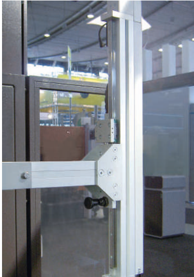
Electromotive VST 2015 with recirculating ball bearing guide
