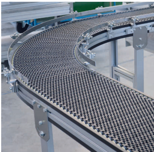
Curved KMF-P 2040 with 90° curve and adjustable side rails
