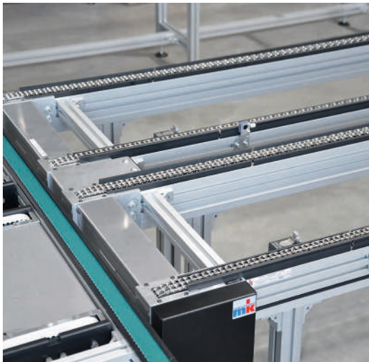
Dual-lane KTF-P 2010 with 80° C temperature resistance
