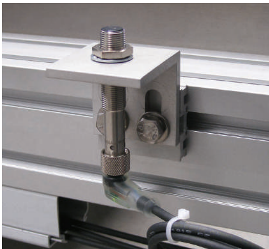
Initiator holder made from aluminium angle bracket
