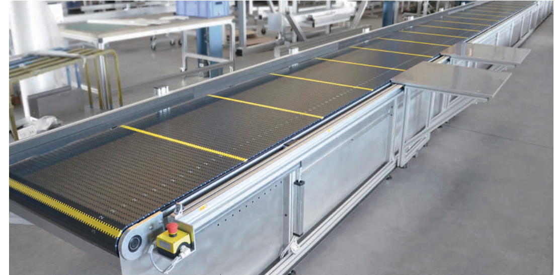
MBF-P 2040 with optical lane separation and workstation tables for manual movement on the line
