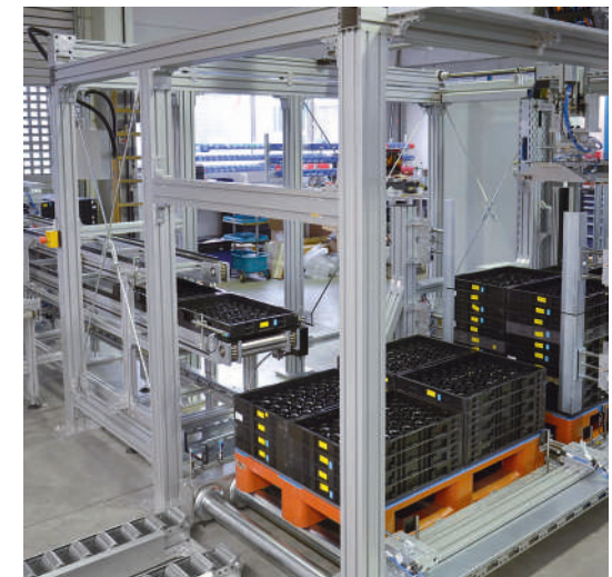
XYZ handling gantry for stacking and unstacking product pallets and euro pallets
