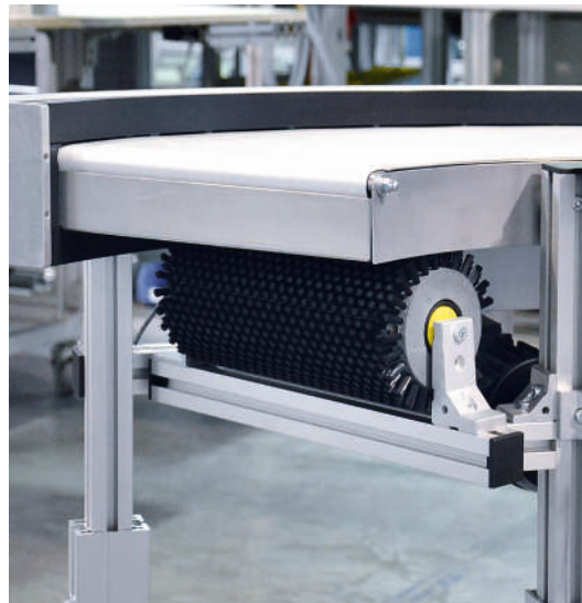
Wiper brush, rotating, mounted at the end of the conveyor
