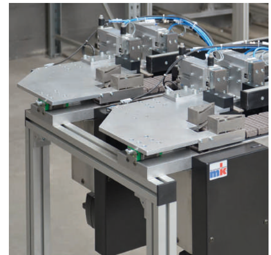
Two-track feed for machine loading. The separator can be adjusted for various diameters using a recirculating ball bearing guide
