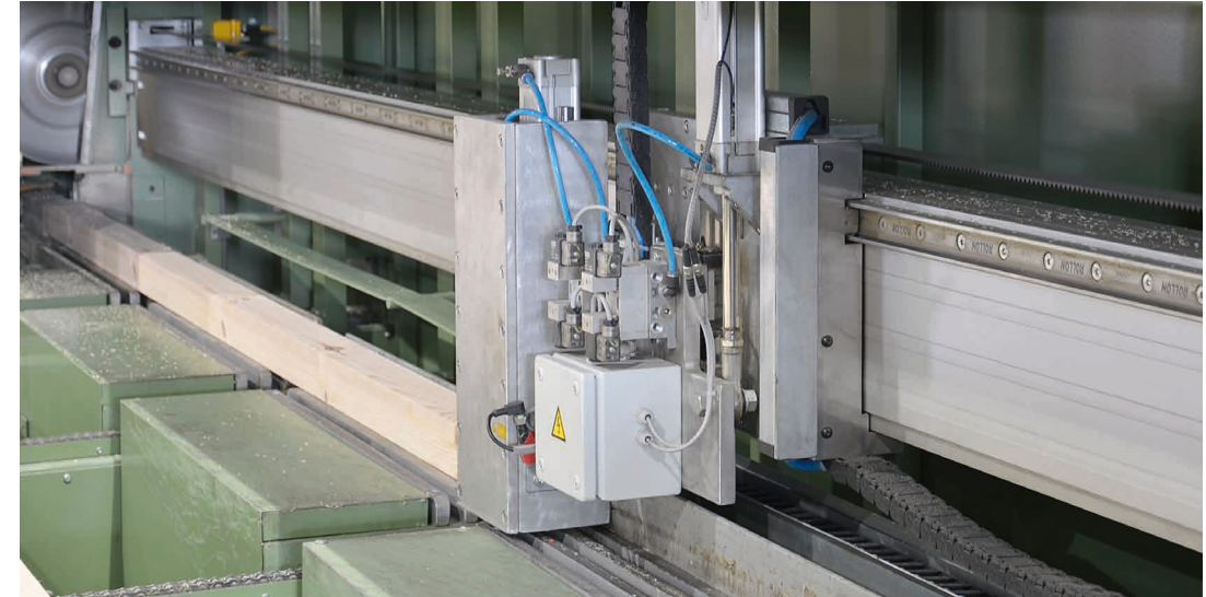
LZR Series 60 linear module based on the mk 2060.07 profile with track rollers and rails from Rollon
