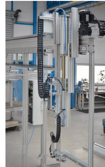
Gantry stand with telescopic gripper unit
