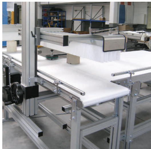
GUF-P 2000 with integrated adjusting unit (VST 2011) for height adjustment of the wiper brushes
