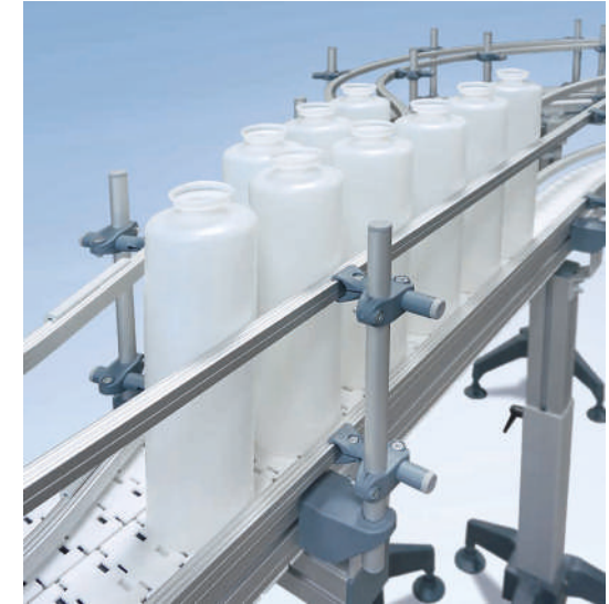
Versaflex SBF A08 with height and width-adjustable side rail
