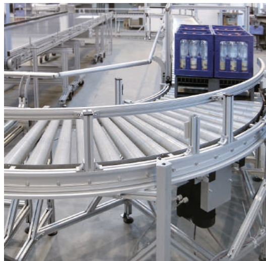
Driven curved roller conveyor RBT-P 2255 90°
