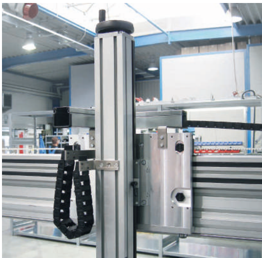
Base LZR 2005-38.44-30 with side roller carriage on foamed combined profile as gantry, with support rollers for torque loads and manual VST 2011 as Z axis
