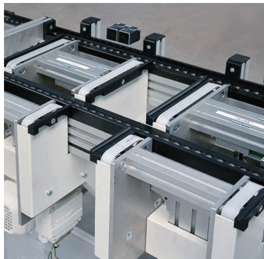
Lift-and-transfer conveyor with coupled drive and central stroke unit for bridging very short transverse sections
