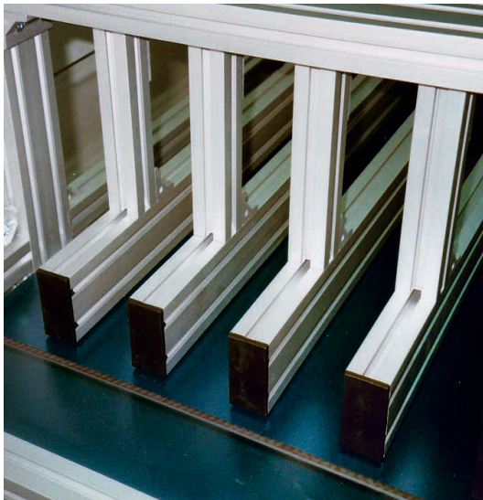
Multi-line, adjustable side rail in gantry arrangement
