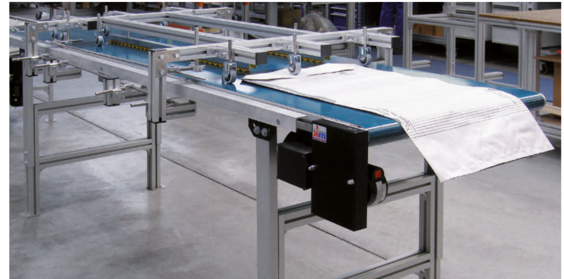
GUF-P 2000 with mechanism for folding and setting up paper bags upstream of the filling process
