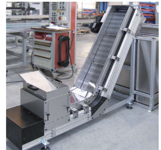
KFS-P 2040.86 for hot product with resizeable supply reservoir
