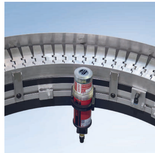
Special flat top chain conveyor with a width of 205 mm with side rail SF 2.1 and lubrication station
