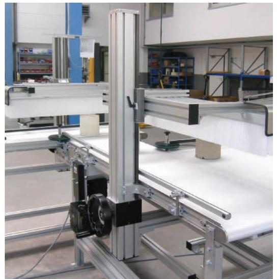
System mk 2011 adjusting unit for brush cantilever
