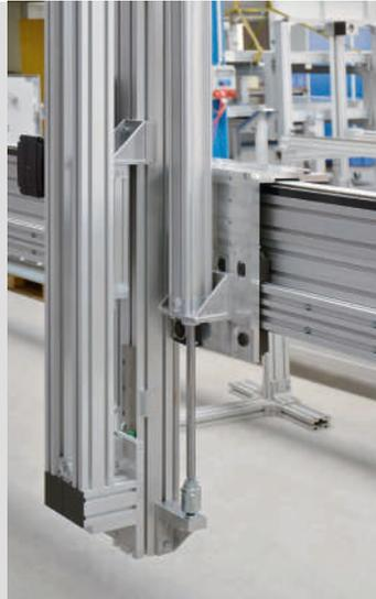
Horizontal axis with foamed combined profile for reinforcement
