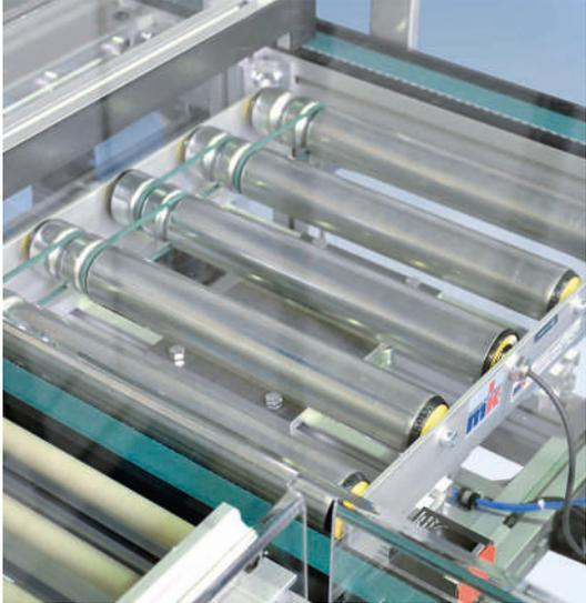
Drive roller conveyor RBM-P 2255 as lift-and-transfer conveyor
