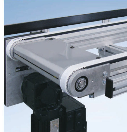
Timing belt conveyor ZRF-P 2010 with head drive AC and side rail for extra-wide products
