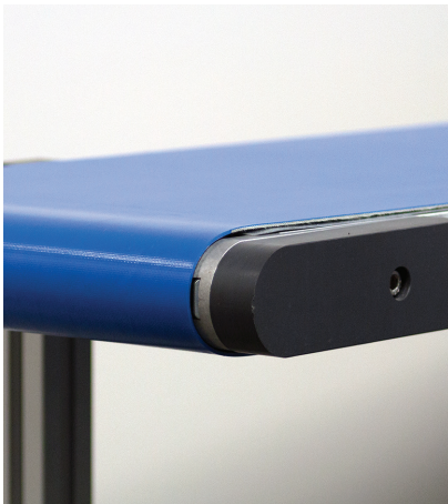
Friction drive conveyors rely on the friction between the drive drum surface and the underside of the belt to propel the belt forward; as shown in this example.
