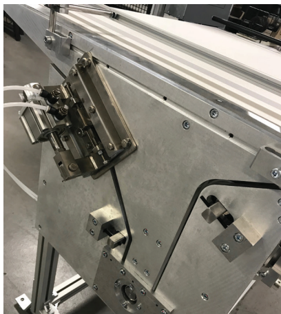
An example of a pneumatic style automatic belt tracking system on a mid-drive conveyor. This conveyor also features micro-transfers at the ends (not shown).
