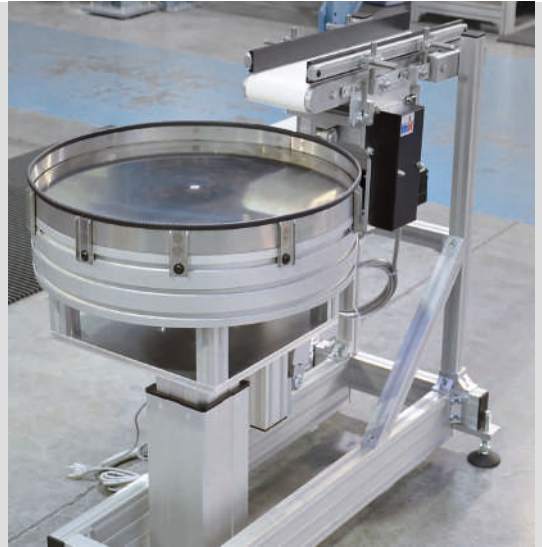
Rotary table with timing belt drive and belt conveyor, all with electrical height adjustment using the telescopic column
