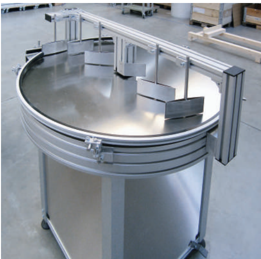
Rotary table with friction belt drive
