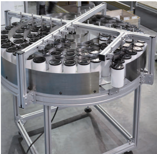
Rotary table with additional custom add-on
